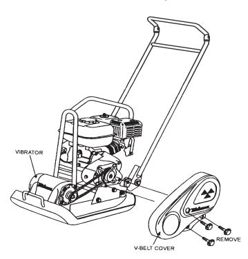
Figure 8. V-Belt Cover Removal
